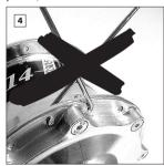
Spokes must not cross directly over the hub cap fixing screws on wheels which are 24" or smaller in diameter!
